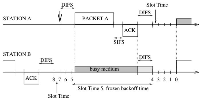
Fig. 1. Example of Basic Access Mechanism
