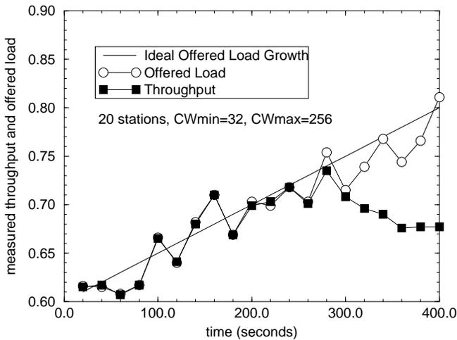
Fig. 3. Measured Throughput with slowly increasing offered load
