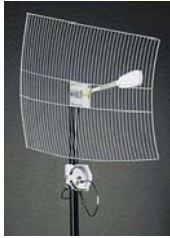
24-dBi Directional Antenna with Up/Down Converter on Mast
